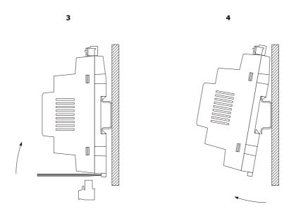
To re-install the EVD HP first press the DIN rail clip fully in.
