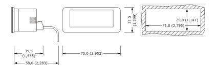
To be installed on a panel with snap-in brackets provided.
