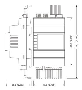
Installation is on a DIN rail  $35.0 \times 7.5$ mm ( $1.377 \times 0.295$  in) or  $35.0 \times 15.0$ mm ( $1.377 \times 0.590$  in), in a control panel. The pictures below show how to install the EVD HP.
