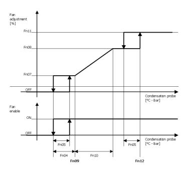
In this mode, parameter Fn13 (external fan pre-ventilation time) is also activated to avoid the compressor starting up at a condensation temperature that is too high. Depending on this parameter, the fan is activated for a time equal to Fn13 before the compressor is switched on and the fan speed is proportional to the condensation temperature. During this period, the fan is set to minimum speed if the regulator requests cut-off.
