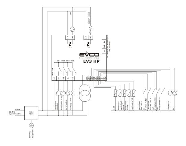
If using triac digital outputs, we recommend connecting a noise filter. The heat sink might reach very high temperatures, do not touch it.
