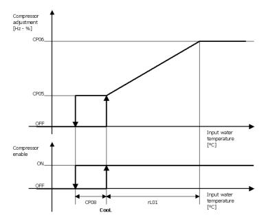
For ON-OFF adjustment, the cut-off delta must be set to 0 and there will be only one adjustment step, as shown on the diagram below.
