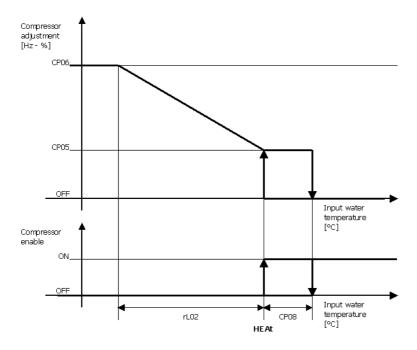
For ON-OFF adjustment, the cut-off delta must be set to 0 and there will be only one adjustment step, as shown on the diagram below.
