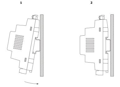
To remove the EVD HP, first remove any plug-in screw terminal blocks fitted in the lower part, then, using a screwdriver, loosen the DIN rail clip, as shown in the pictures below.
