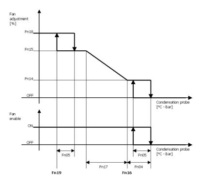
The diagram below represents the ON-OFF adjustment in hot mode.
