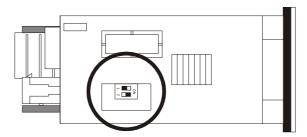
When using EVD HP, place micro-switch 1 in position ON.
