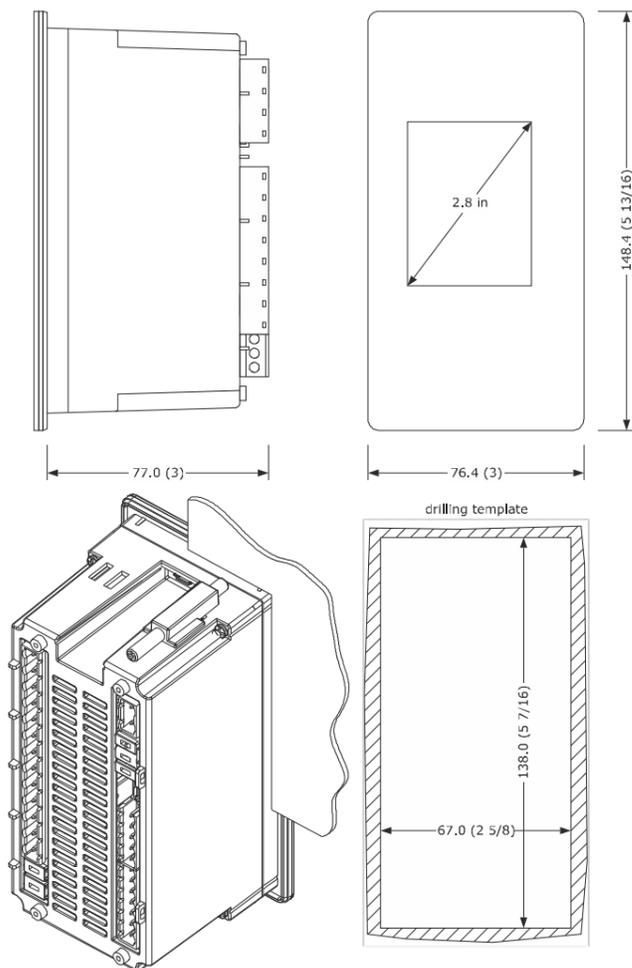
The tolerance of the measurements of the drilling template is +0.2 -0 mm.
