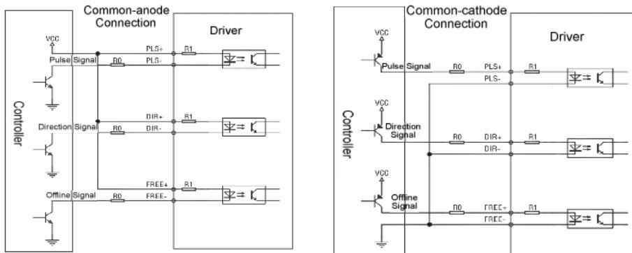
**Control Signal Wiring Diagram**
