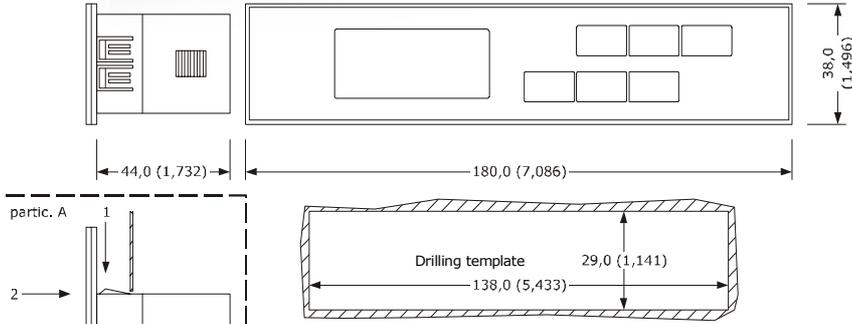
To make easier a possible removal of the device, slightly bevel the longitudinal inside edges of the drilling template before the installation (det. B and C).
